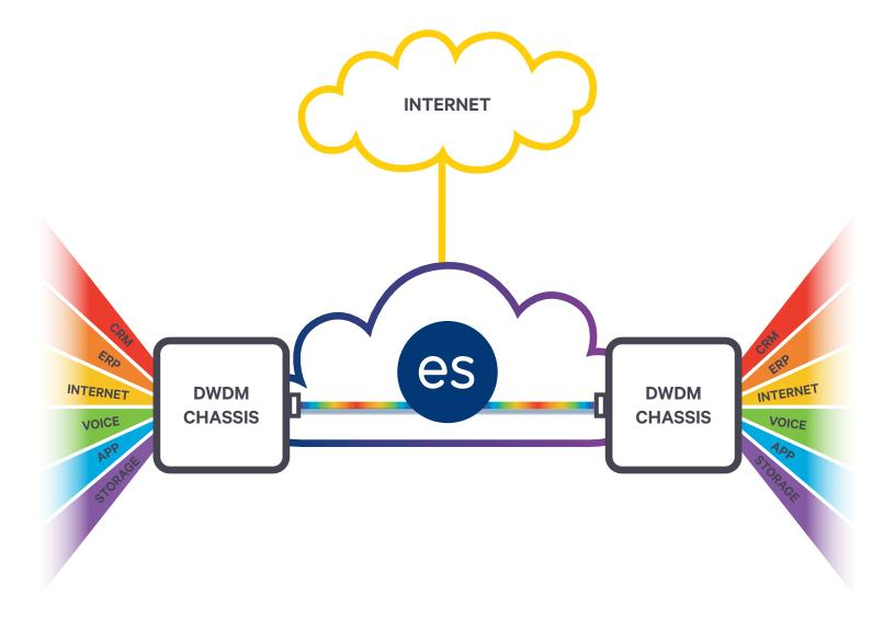
Dedicated Dense Wavelength Division Multiplexing (D-DWDM) is an optical, multiplexing technology used to increase bandwidth over existing fiber networks. It works by combining and transmitting multiple signals simultaneously at different wavelengths on a single fiber strand.
